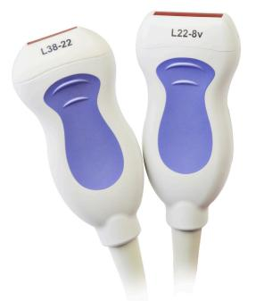
Kolo Medical is a leader in next generation semiconductor (silicon) ultrasound transducer technology. Kolo's Silicon Wave transducer technology offers a practical alternative to PZT transducers for extremely broad bandwidth and high frequency imaging applications. These transducers provide unparalleled imaging performance for pre-clinical imaging, including mice and rats, and for other superficial imaging applications.
