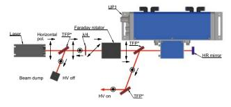
TFP – Thin film polarizer, for instance our standard products: 420-1258UHT, 420-1256UHT or 420-1248UHT.
