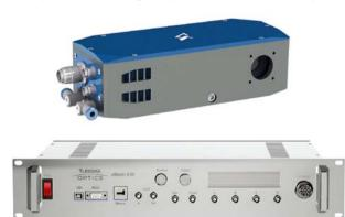
MP1 pulse picker consists of built-in fast driver and a Pockels cell. This unit is able to select pulses at up to 600 kHz rate. MP1 requires sync pulses from the laser for the driver control or can be used with pMaster 4.0H generator. In setup with pMaster 4.0H generator can be synchronized for single pulse picking from max 30 MHz repetition rate pulse train.
