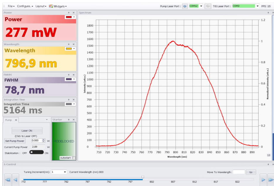
Widget-based software screenshot for the TiF family of lasers with integrated spectrometer ("Auto" package)
