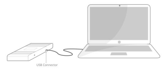
IMPORTANT: Remember to unplug the external power from the spectrometer before connecting the USB.
