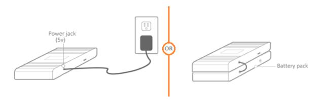
IMPORTANT: Remember to unplug the <u>USB cable</u> from the spectrometer before connecting the external power, otherwise it will not work.
