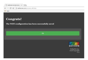
NOTE: Now the spectrometer has added the WIFI configuration to its network list. Next reboot it will try to connect to the first network in the list and if it fails, then it will try with the next one and so on.
