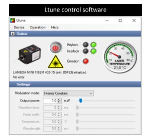
All operating parameters can be monitored and controlled from a PC using the Ltune laser control software for Windows. Alternatively, the laser can easily be controlled from your own application software. Please refer to the user manual for a detailed description of the communication protocol. You can find downloads on our website
