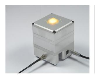
The ArcSphere-50-Hal is an integrating sphere with internal halogen light source for diffuse reflection VIS/NIR measurements. It has an internal diameter of 50mm, a sample port of 10mm with a sapphire window, and an SMA fiber connector to connect to the spectrometer
