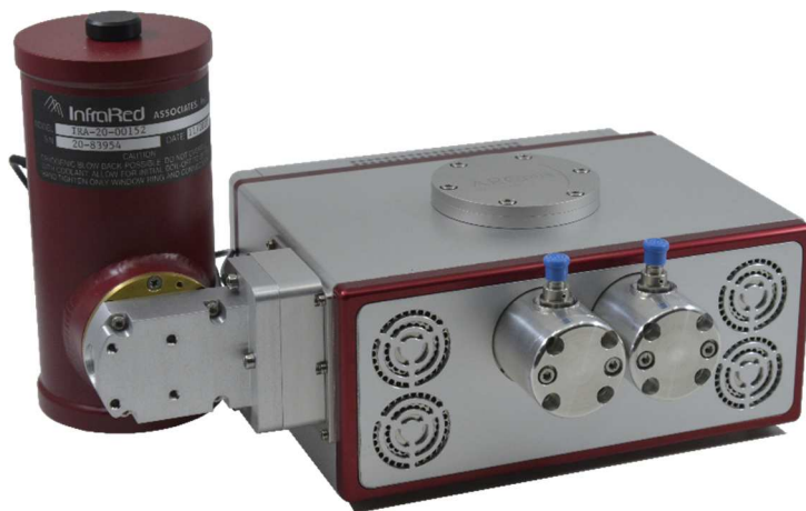
FTMIR-FC unit mounted with an MCT detector cooled by LN2
