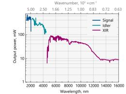
*Fig 1.* Typical output PT277-XIR tuning curve. *The actual tuning curve might differ from presented here.*
